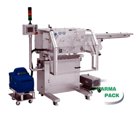
The function of LFOS-12 booklet outsourcer is: pre-folded booklets, which are manually placed on the conveyor, are sucked by vacuum sucker on the rotary axis are transferred forward. When a bottle is coming, the sensor sends a signal to PLC and PLC instructs the glue dispenser to spray glue. Then the vacuum sucker press booklet on the cap and the booklet stacking process is finished.
