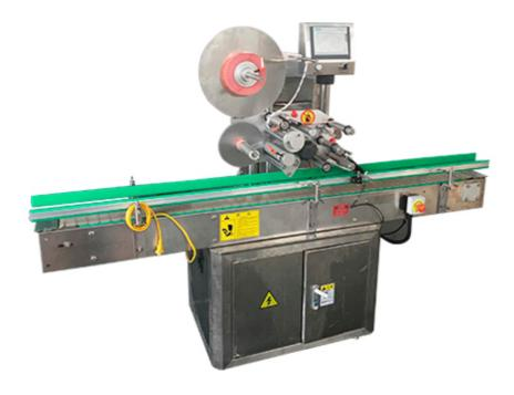
For standing firm circular cylindrical objects, semicircular labeling, the use of horizontal transmission, horizontal labeling way to increase stability, improve the labeling efficiency.
