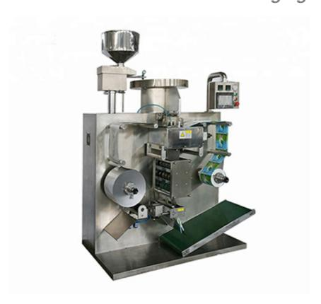
This machine is suitable for the automatic bi-al foil sealing of capsules and tablets or balls for the pharmaceutics, chemistry and food-staff industry. The package can be airtight and can avoid the light, and also can seal the capsules bi-plastically.
