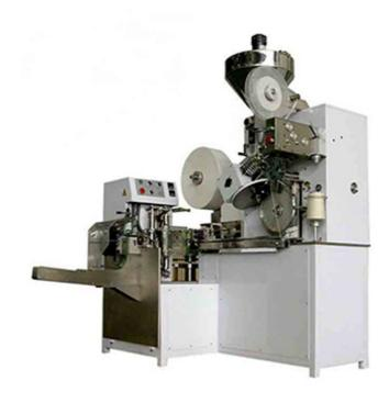
Automatic Teabag packing machine model DXDC8iv is newest generation machine whose functions include filling, heat sealing, threading, labeling and overwrapping. This machine adopts sealing pads to replace the sealing rollers on old machines. The new system greatly improves machine's flexibility for different packing materials and will supply best teabag package. Many kinds of packing material will get good performance on this machine such as paper/P.E, Plastic/P.E, Plastic/P.E etc
