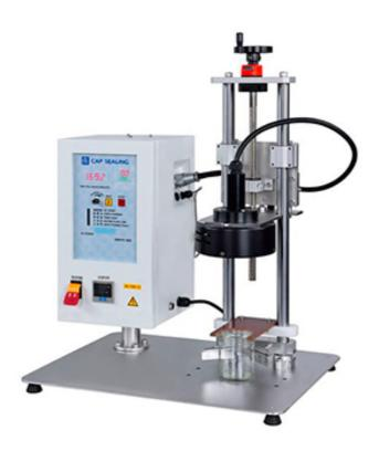
Specially designed for uncapped bottles, it's suitable for small enterprises, manufactories or labs for sealing various vessels in small quantities; it is light in weight, high in efficiency and easy to operate. It is used for sealing various types of bottles. We can customize different diameter's bottle. This machine does not contain air compressors, and must be self-prepared with an air pressure of 5 kg/cm2 or more.
