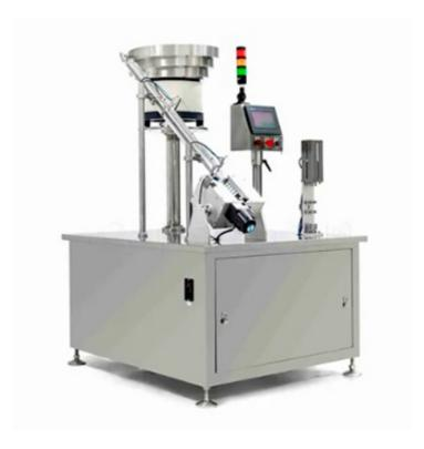
CED-S10A semi-automatic effervescent tablet tube filling machine is a highly efficient packaging solution designed for the pharmaceutical, food and daily chemical industries. The equipment is suitable for counting, filling, sealing and other packaging processes of products such as milk tablets, effervescent tablets and vitamin tablets. It has the characteristics of easy operation, high degree of automation and accurate counting.
