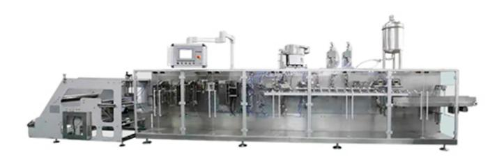
BHD-240SC is specially designed for stand-up bags with standard suction nozzles. It can make larger bag sizes and filling volumes, with a maximum filling volume of 2000ml. The suction nozzle can be designed as a straight suction nozzle or an angled suction nozzle. Often used to package large quantities of laundry detergent, milk, juice, and detergents.
