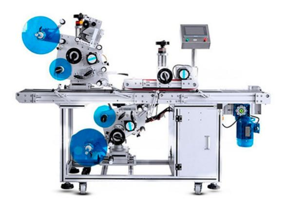
This labeling machine is designed for labeling stickers on upper and bottom flat surface at the same time, this can improve working efficiency greatly and reduce production error. It is widely used in daily chemical, cosmetics, food and beverage industries.
