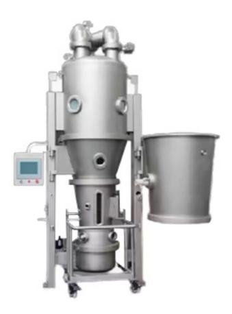
FBM Series Fluid-bed Multi-processor is added bottom spray on the base of FBG series Fluid-bed Granulator, thus can realize drying, granulating and bottom spray coating on one machine, and with function of mixing raw material, granulation, dying and coating for granules or pellets. The equipment is PLC auto controlled and well satisfies with the current GMP and the National Pharmacopoeia.
