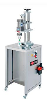
The container cap closing equipment is semi-automatic capper. It is suitable for object container with plastic screw caps.
