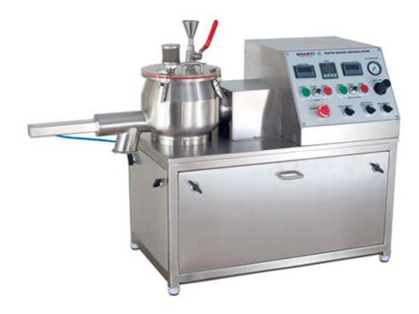
The SHAKTI Pilot Scale High Shear Granulator and Mixer is designed for efficient and homogenous wet granulation of powders to form a medium to high density granule. It is mainly used in R&D or F&D facility for the wet mixing of the pilot batches. Basically it consists of a Bowl, Impeller & Chopper assembly.
