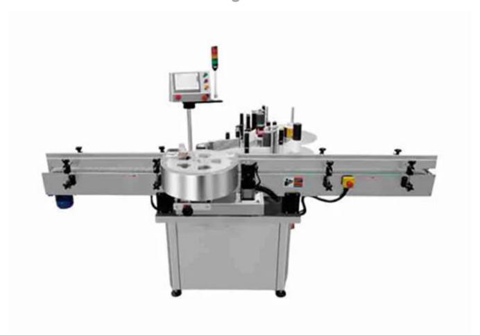
Bottle feeding  $\rightarrow$  astrolabe clamping bottle  $\rightarrow$  batch number printing  $\rightarrow$  positioning labeling  $\rightarrow$  testing and dismantling  $\rightarrow$  finished product. This equipment is suitable for labeling large round bottles made of glass, plastic, metal, etc. (such as large infusion bottles, penicillin bottles, eye drops, syrup bottles, beverage bottles, etc.).
