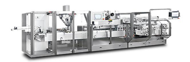
Masta is a high-end cartoner, which is optimized for producing top-end products and increasing user convenience. This model operates in intermittent motion with minimal noise and vibration by using belts in major drives. Its compact and premium design is differentiated with other model that proves Hoong-A's advanced technology and development.
