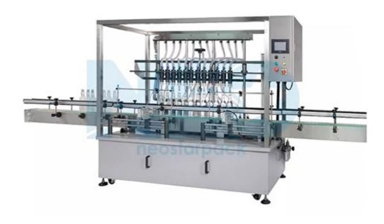
12 Nozzle over-flow liquid filler FL4670 overflow filler is built to meet the requirement of consistent filling level. It is especially suits for foamy, flammable, or corrosive liquid filling. Moreover, with PLC and HMI control system, all filling parameters can be set and monitored in screen easily. Number of filling nozzles or other options like product supply pump is available according to different requirement. It is absolutely the best choice for your company.
