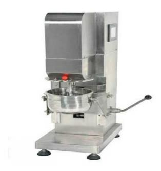
GHL10 High Efficient Wet Mixing Granulator is used the most common international granulation method. The granulation process, granulation by mixing the two processes to complete in the same container. Powder materials are in a fixed conical container, stirring the mixture with the diced knife blade opposite effect in that the powder was dispersed collision state of semi-rolling flow, and achieve full hybrid, with the injection of adhesives, so that powder materials gradually mixed.
