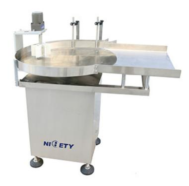
Operators put the upwards bottles on the turn table, bottle feeding system deliver the bottles to the conveyor automatically and orderly.
