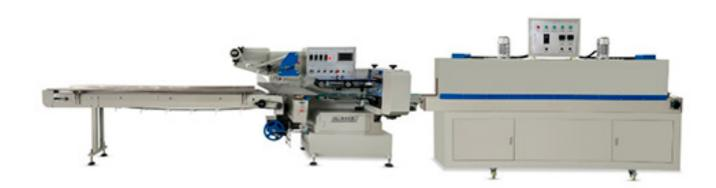
Full servo pillow type packing machine use a conveyor fed automatic operation. Soft feed conveyors carry products into the system and places them inside the folded shrink film. An adjustable sealing arm raises and lowers as products move through the system. Once sealed, the closed pouch is then moved into a shrink tunnel, shrinking and tightening the film.
