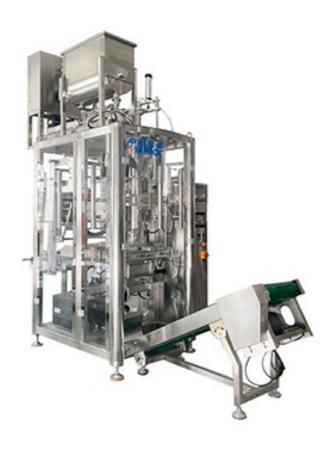
This unit machine is special design for packaging liquid and solid mixture product into plastic bag. The machine have the function of automatic bag forming, Solid product weighing, Liquid product measuring and filling. With optional function of exhausting the air inside the bag and then sealing the bag. The machine also have color ribbon for date printer for coding of expiry date and production date.
