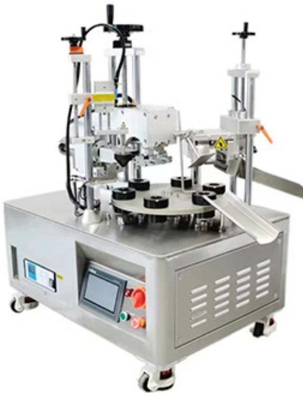
The semi-automatic ultrasonic tube sealing machine with a 10-position rotary table is designed for efficient and reliable sealing of soft tubes. This model is particularly suitable for industries such as cosmetics, pharmaceuticals, food, and household chemicals, where precision and consistency in sealing are crucial.
