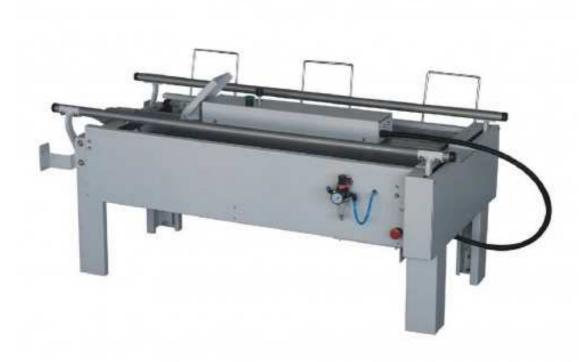
Case erectors and case cartoners are case equipment which automatically forms corrugated cases. A stack of corrugated blanks are knocked down and placed into the machine. The blanks are pulled out of the machine one-by-one and formed into cases. The newly formed cases are sealed at the bottom with tape or glue.
