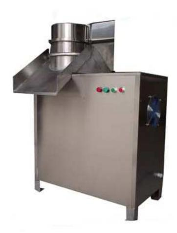
The machine is used for pharmaceutical industry, foodstuff industry, drinking reagent industry, chemical industry; solid industry. It can make the mixed raw material become the needed granule. Particularly it is suitable for raw materials with high viscosity.
