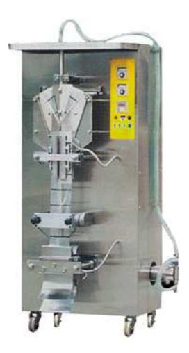
This machine is widely used to pack liquids of low and high viscosity such as pure water, milk juice, beverages, soy sauce, vinegar and wine, etc. It can automatically sterilize the film with violet ray, form the bag, print the code precisely fill the product and seal & cut at one time. It used as single lay PE file and co extrusion film.
