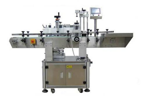
This machine is applied to label the self-adhesive label on various round bottles or containers. It has accurate positioning function, high-speed labeling front and back at the same time. This machine is widely used in pharmaceutical, foodstuff, and beverage, cosmetic, chemical and etc. industries.
