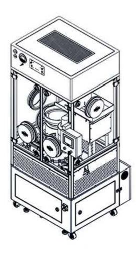
The Model CP-20N Automatic Vial Capper is designed either to couple with a vial filling & stoppering machine to complete an in-line operation or to operate independently. It is a reliable cap closing machine to apply aluminum seal to serum vial at speeds up to 120 units per minutes. It operates on an intermittent motion principle and features readily adjustable rollers to perform the sealing function.
