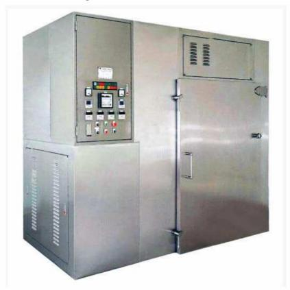
The Drying object either powder or granules is placed on the drying grays which are made of special screens or punch hole plates and covered around by filter cloth.
