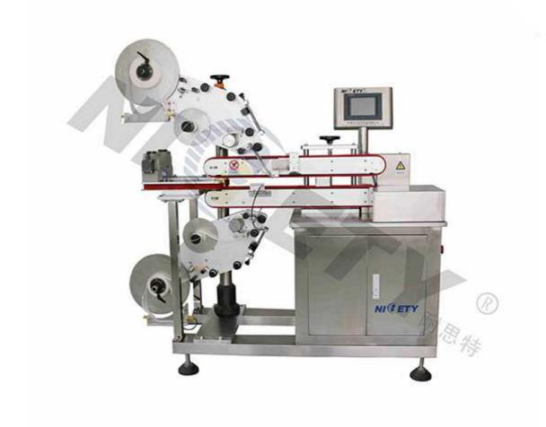
The equipment is used for pasting sealing label on the carton.
