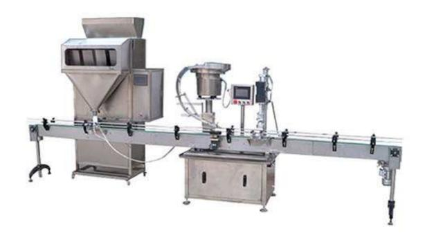
Automatic granule filling machine production line
