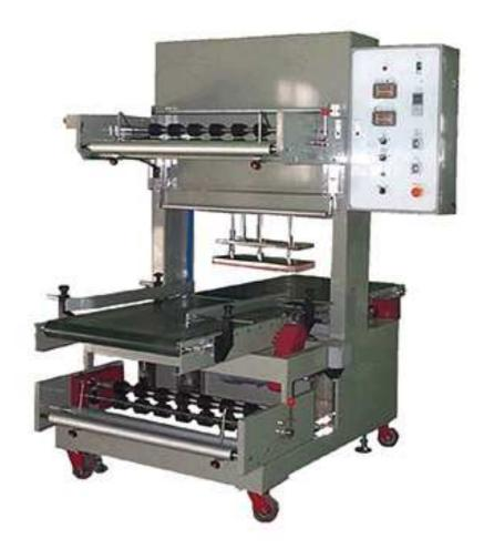
SA-117-V inline-type sleeve sealing machine is suitable for products in one tray pack, single carton or some simple collections of large products. Available with transparent PE shrink film (each Top and Bottom film cradle) OR printed PE film (only Top film cradle) Its speed could up to 12 PPM depends on the product dimensions.
