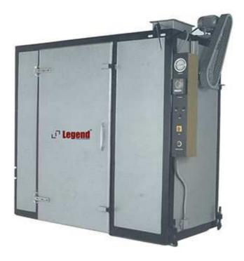
A tray Dryer is an enclosed insulated chamber in which trays are placed on top of each other in trolleys. Tray Dryer are used where heating and drying are essential parts of manufacturing process in industries such as Chemicals, Dye stuff, Pharmaceutical, Food Products, Colours etc. The material to be dried either wet or solids are placed in the trays. Heat transfer is by circulation of hot air by electric heaters or steam in radiator coils.
