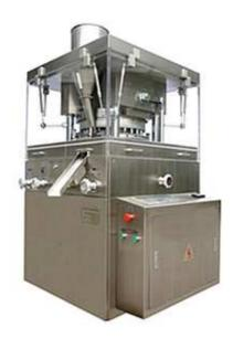
The machine is a double pressing automatically revolving piece-pressing machine which could make grain be pressed to be round pieces, be carved characters, special shapes and double color piece prescription. It is mainly used in manufacturing piece prescription for pharmaceutical industry enterprises like chemical, food, electronics.
