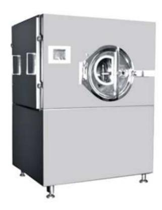
BG Series coating machine is a multi-function coating facility mainly supplied by pharmaceutical and foodstuff industries for sugarcoating or film-coating process.
