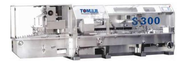
The new series cartoning machine built with "BALCONY" design, allowing the mechanical working parts separated from the packaging area. It respects the present accident prevention maintenance and hygienic laws. The machine works with intermittent motion and with electric synchronisms controls, PLC and touch display control system functions recall-able; it is possible memorizing 100 menus with relative data for 100 different productions.
