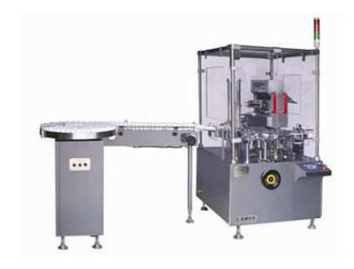
This machine is suitable for cardboard case packaging of medicine bottles (round, square), cosmetic, and food and so on. It consists of direction folding (1-4 folds) and feeding equipment, cardboard case forming and feeding, batch number printing, sealing of case tongues at both ends ect. The whole encasing process is finished automatically. It can be added hot-glue machine.
