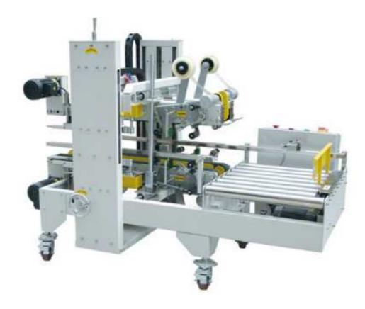
Corner sealing machine (turn type) carton by the front of the sealing machine in the middle of the upper and lower sealing, into the 90 degree corner machine, push the box by pushing the corner box sealing machine, and automatically sealed up and down four corners of the box, fast, smooth.
