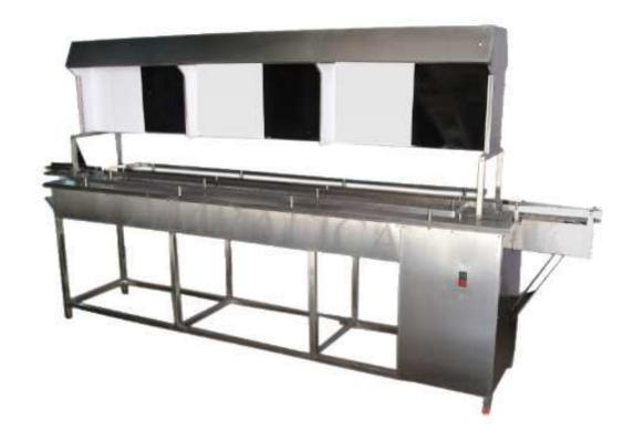
On-line filled & capped containers are fed in to machine via single conveyor divided in equal quantum in further movement on two lines for visual inspection by operators. Black and white background helps them to inspect the bottle visually. On inspection the bottles are placed on center conveyor for outlet.
