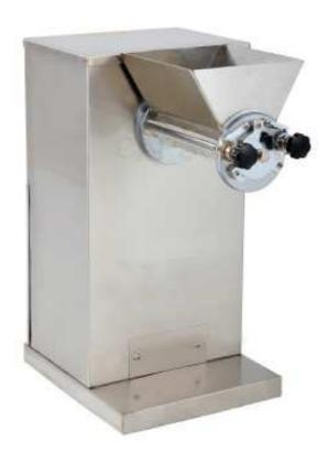
This machine is used mainly in such trades as pharmacy, chemical industry, food, pottery and plastics extensively, making moist powder material particle. Make cylinder swing reciprocatly, extruding material from screen mesh for granulation. It also can be used for crushing the agglomerate materials into small granules directly.
