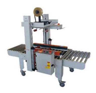
It can be wired or stand-alone operation, manually fold up and down the lid, together with the middle of the tape sealing
