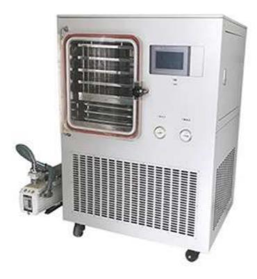
BFD-100P floor model Freeze Dryer (Lyophilizer) fit lab research or small scale pilot production, config with 6 material trays at 360\*480mm, all shelves with heating and freezing function, during in freeze drying process, the shelves temperature could flexible program from -50C to +70C with accuracy of 1C.
