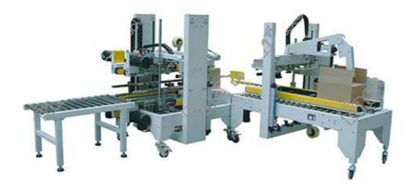
Fully-automatic box folding & sealing machine is used to fold and seal boxes/cartons automatically. It integrates a folding & sealing machine for upper side and a sealing machine for four sides.
