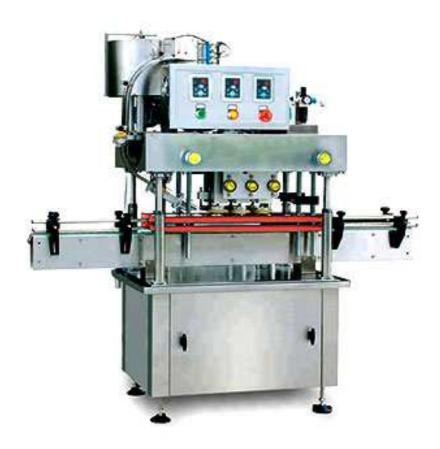
In-line belt wheel capper with a automatic caps feeder and 6 spindles. This machine is a universal capping machine in order to face the current diversity characteristic of the capping machines.
