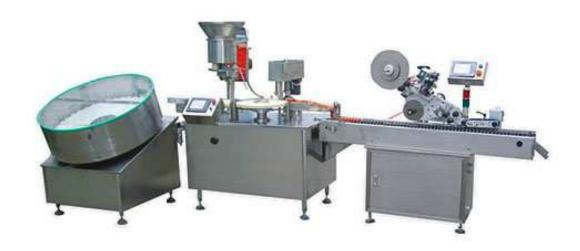
This unscrambler filler capper sealer is mainly designed for the unscrambling, filling, capping and adhesive labeling of plastic bottles. And its main parts are unscrambler, filling machine, automatic capping machine, and adhesive labeler.
