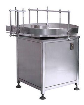
Motor drive send bottles of wheel rotation, From storage bottle tray into the bottle of rotary bottle after dialing bottle device Article will bottles lined up automatically into the guide, the guide bar again into orbit . The bottle to the photoelectric counting bottle machine conveyor belt connection place, into the conveyor belt for the number of electronic machine automatically
