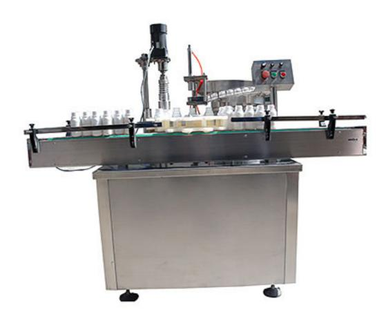
Automatic capping machine use frequency conversion control, for all kinds of bottles auto capping. Reasonable design, compact structure, screw cap does not damage the cap, high efficiently, stable and reliable, long service life, using SS304, meet the GMP. Widely used in pharmaceutical, food and chemical industries.
