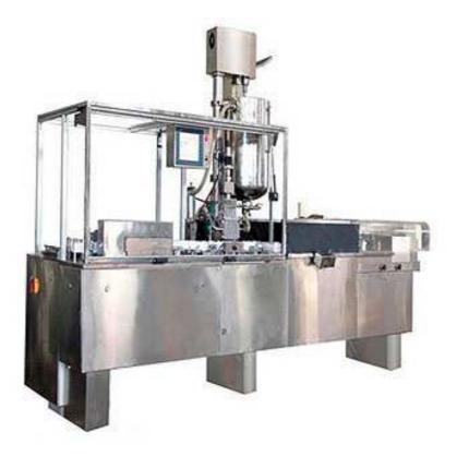
BGZS-9A High Speed Suppository Filling and Sealing Production Line with output 16000-22000 pcs/h which is made up of high speed suppository belt forming system, filling machine, cooling machine and sealing machine. PLC programmable control and human-computer interface operation the unit is simple to operate and with high automaticity.
