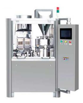
Automatic capsule filling machine is Small size, low noise with PLC and touch screen control, operates steadily and reliably.
