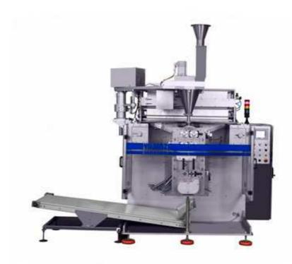
The rectangular shaped bags as 'sachet type' (that are glued in their four sides) are produced in the machine which has the property of multiline production. Depending on the size of the package, it can work 10 lined. Its capacity can reach 500 pieces/min and it can handle high capacity of production power with one machine. With proper dosaging unit, it can pack different products such as powder, granulated, liquid and wet wipes.
