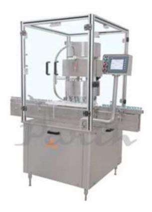
Automatic VIAL Cap Sealing Machine is versatile, self-supported on stainless steel leg with height adjustable adjustment system. The machine is precision built on sturdy welded MS frame completely enclose in stainless steel sheet and doors are providing to facilitate the servicing of machine.
