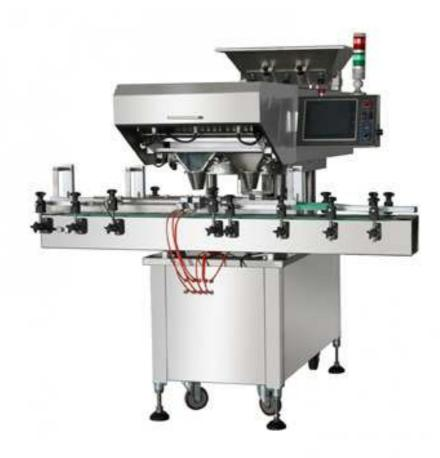
A newly improved Softgel counting machine consists of 16 track format with dual filling nozzle. Adoption of new Digital Camera System: CCD technology, the CCD-16 combines unerring accuracy with incredible value. The machine handles a wide variety of tablets, caplets and both hard and soft capsules with different shapes and sizes.
