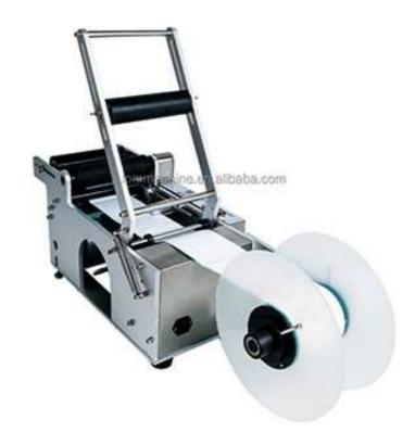
It is mainly used for round bottles, square or special-shaped bottles, and can label with one or more labels, Use servo to label, Stable labeling and high precision, According to the need, install the hot stamping machine, print the production date, batch number and shelf life, etc. Manufactured in accordance with GMP standard. Widely used in pharmaceutical, food and chemical industries.
