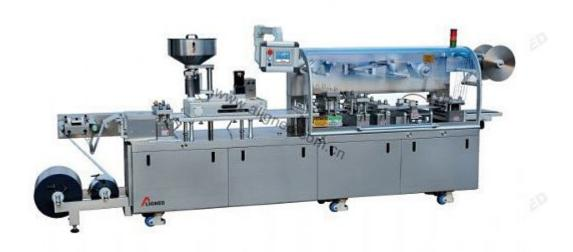
Multi-packing machine - Blister machine DPP260K2 is a compact processing line. With the help of medicines packaged into blisters, followed by coating them perforations and output data.
